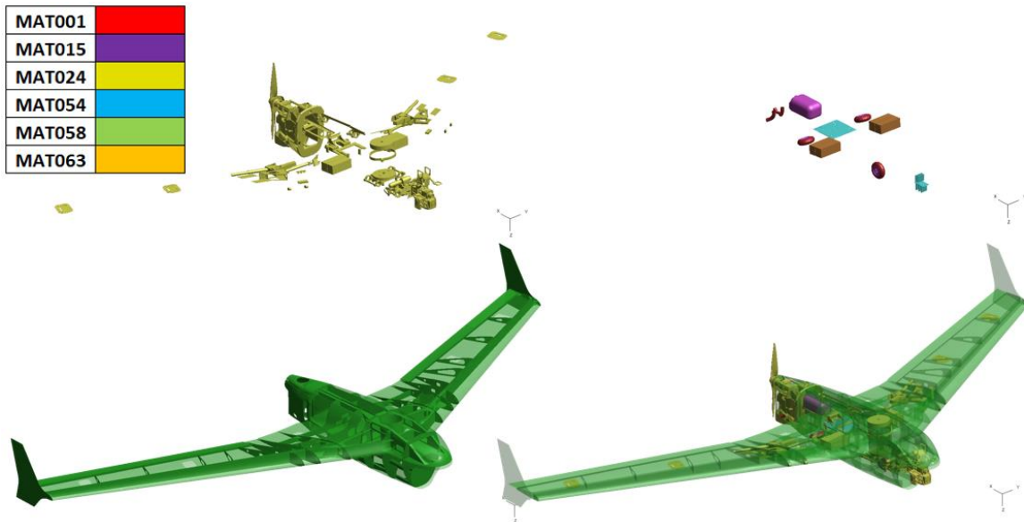
Figure 37. F25 & F55 UAS material models for LS-DYNA solver.
