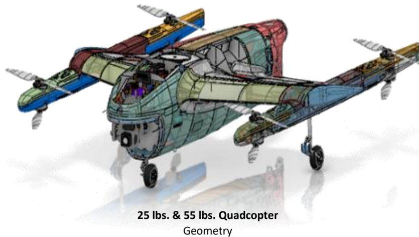
Figure 13. NIAR UAS quadcopter configuration CAD representation.
