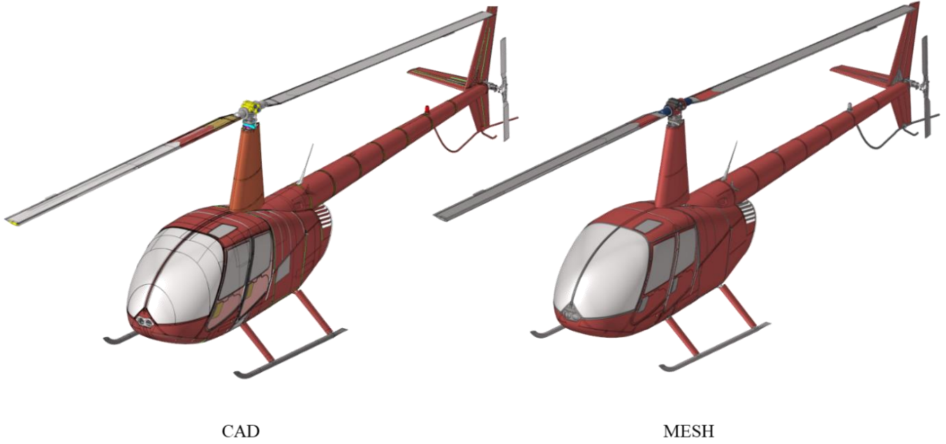
Figure 96. Rotorcraft CAD vs. mesh.
