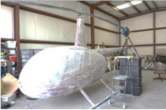
Figure 52. Part 27 Rotorcraft coated for OML Scan.
