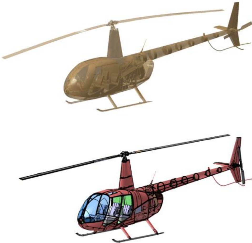
Figure 55. Part 27 rotorcraft 3D scan data vs. CAD model.
