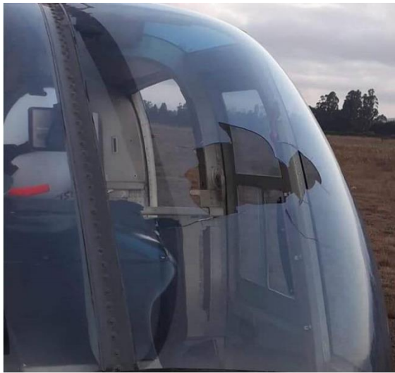
Bell UH-57B. Different helicopter but similar windshield construction (plexiglass). sUAS was a DJI Mavic Air 2, 0.57kg (1.26lbs)
