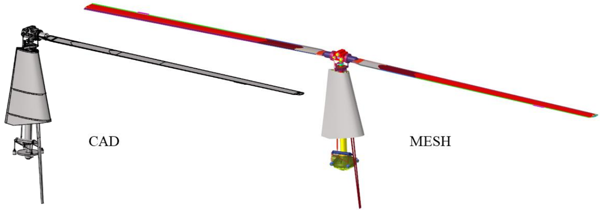
Figure 102. Rotorcraft mast assembly CAD vs. mesh.
