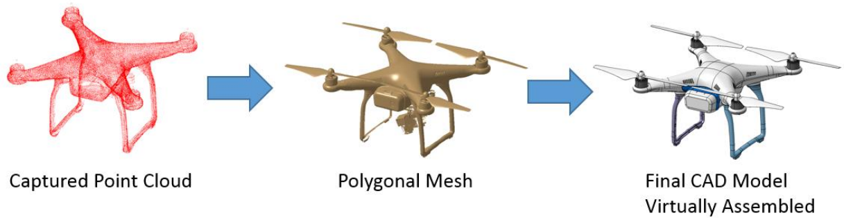
Figure 9. UAS 2.7 lbs. quadcopter CAD model development steps.
