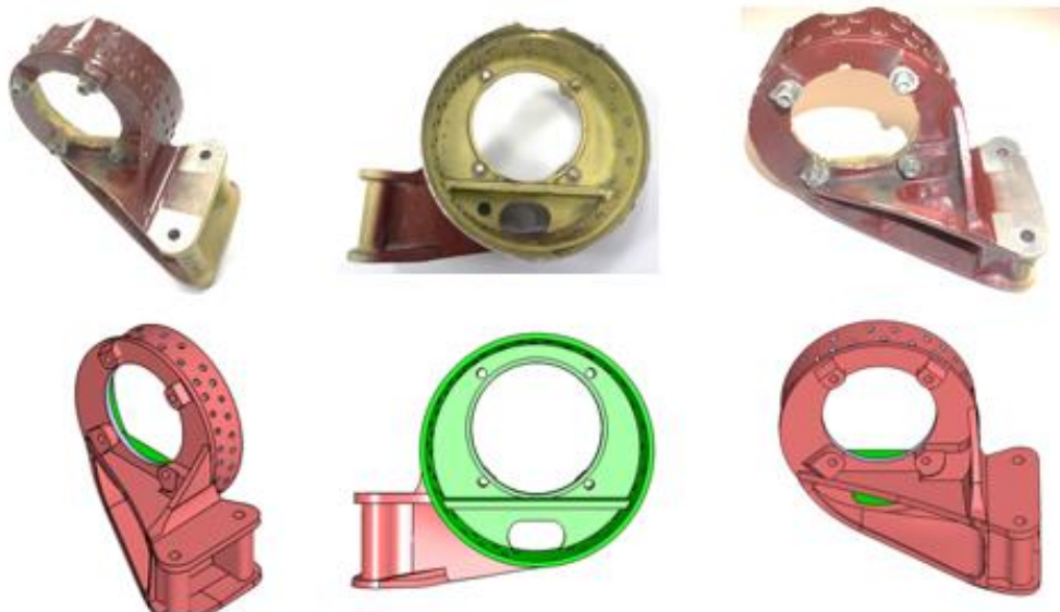
Figure 68. Part 27 Rotorcraft tail cone machined frame.
