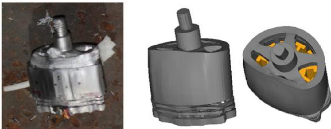
Figure 46. Comparison of the test (left) and simulation (right) projectile damage for motor A impact on 0.25" aluminum panel at 267.51 m/s (520 knots).
