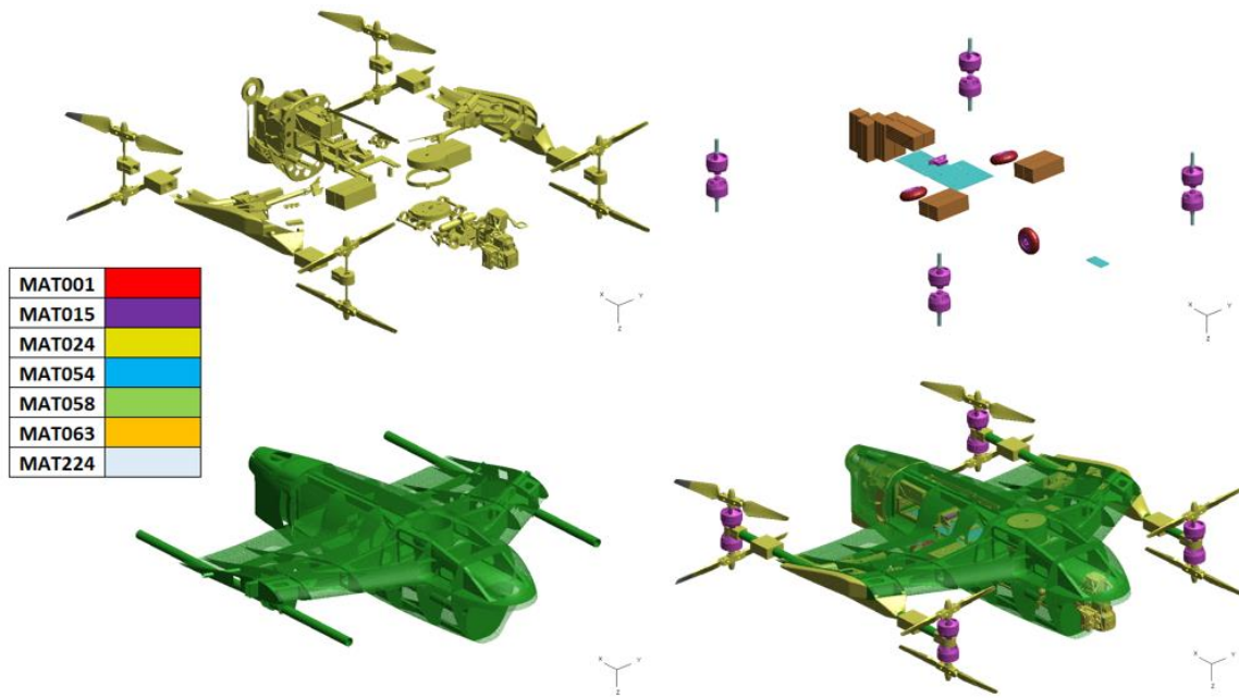
Figure 34. Q25 & Q55 UAS material models for LS-DYNA solver.
