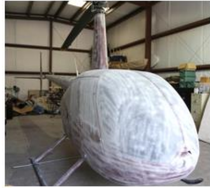
Figure 52. Part 27 Rotorcraft coated for OML Scan.
