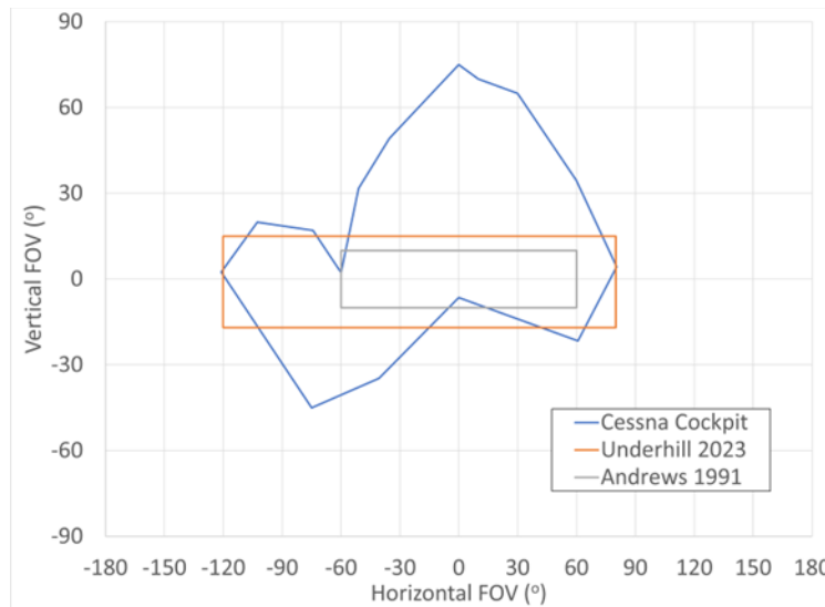
Figure 64. Different standards for ownship Field-of-View.
