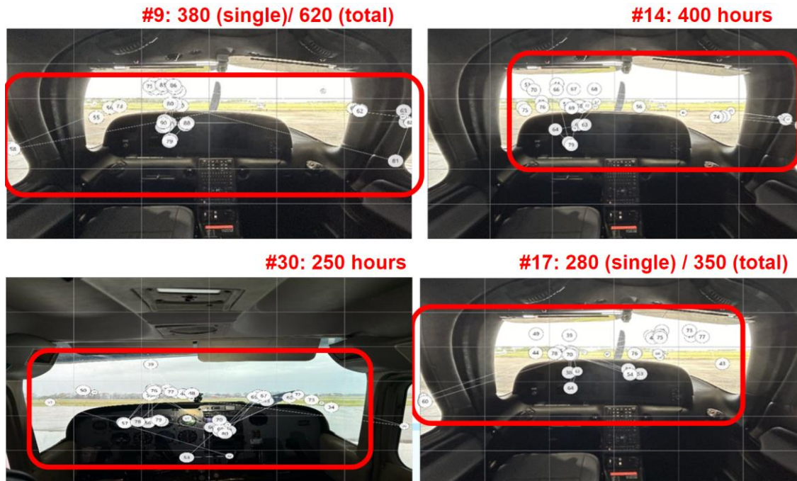
Figure 34. Experience impacts on scan pattern for pilots with more than 120 single engine hours.
