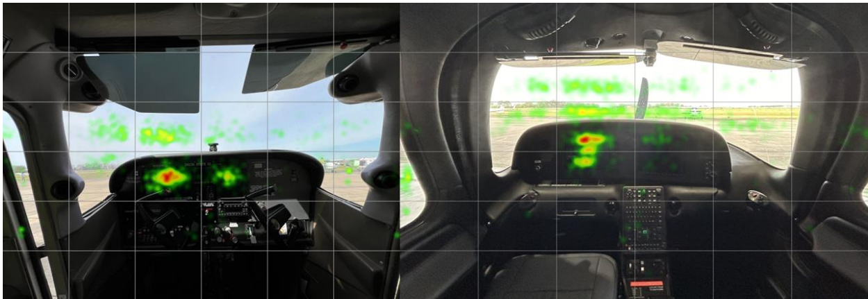
Figure 30. Scan pattern in C172 on left and Cirrus SR20 on right.
