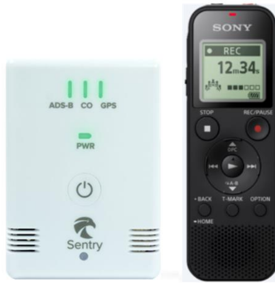
Figure 2. Sentry ADS-B receiver unit and Sony PX-470 audio recorder.
