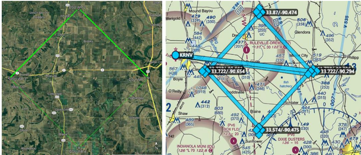
Figure 15. Ownship's diamond shaped flight path for overtake encounters.
