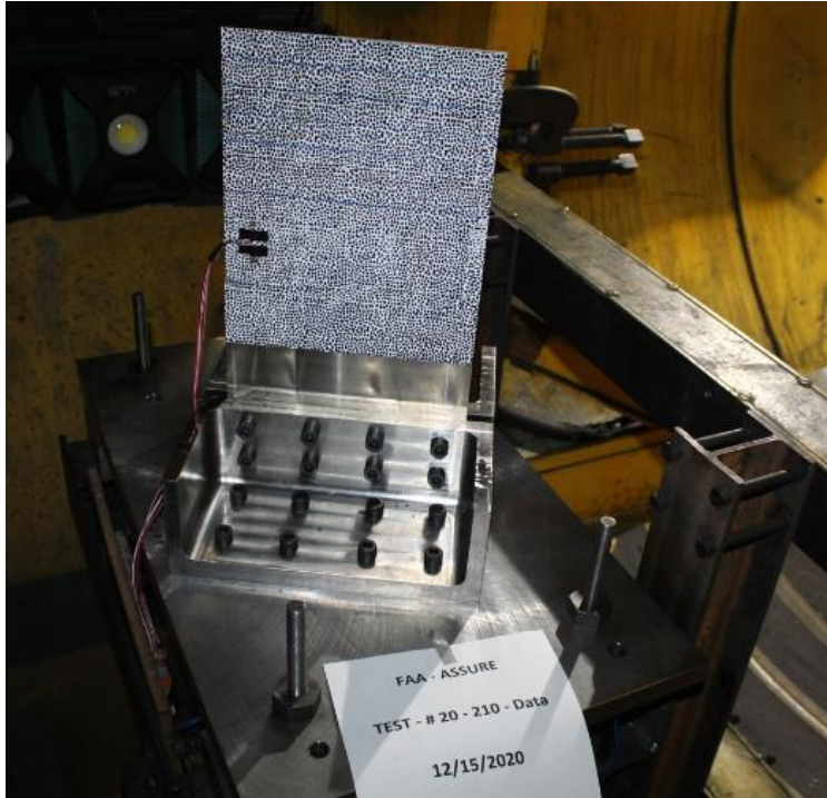
Figure 18. Titanium test article, stainless steel bracket, and tabletop mount.
