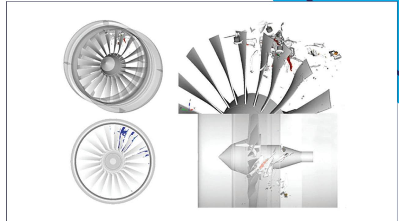
During the simulations these components give appropriate boundary conditions during the ingestion and enable the computation of the expected loads on these parts. This allows for the determination of cases where the greatest energy and/or strain is imparted to these components and enables industry to focus on these cases when using their actual proprietary designs.
