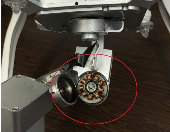
*Figure B - 6 - Camera Separation from Gimbal at the Elevation Motor on Test Article UA17A-10*
