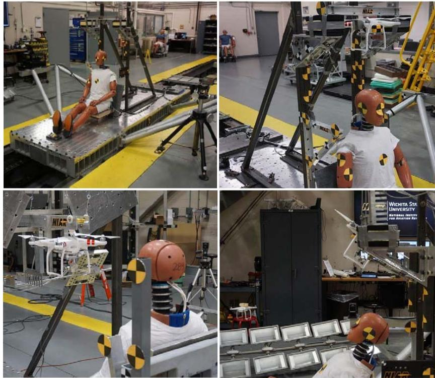
*Figure 3 - Front Left View of Sled Setup (upper left), Vertical Drop Position of Dummy and UAS (upper right), Pendulum Setup for Horizontal Impact Test (lower left), and Dummy and UAS Setup for Angle Impact Test (lower right)*
