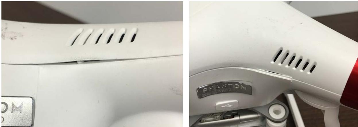
*Figure B - 1 - Buckling on Test Article UA17A-05*
